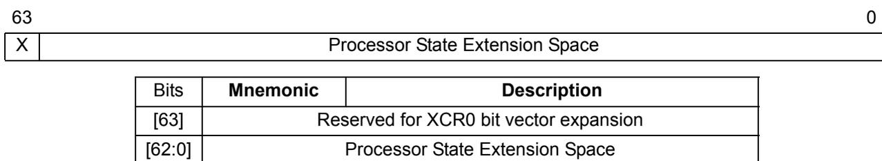
**Figure 1-7. XFEATURE\_ENABLED\_MASK Register (XCR0)**
